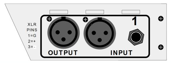
The audio INPUT is a female, 3-pin, XLR connector that feeds an active balanced circuit.
