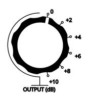
As a result of the dynamics control, the level of the output signal of the device suffers a certain level decrease, this is the case with most dynamics control devices, this is a normal phenomenon. The output signal level controller provides an opportunity to compensate for this signal level loss. To compensate for the output signal level, turn the output signal level control clockwise until the mark on the control knob points in the direction of the desired compensation value.
