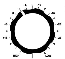
The intervention threshold level, THRESHOLD, determines the signal level at which the dynamics controller starts compressing. The timing of the intervention can be manipulated by the operator by setting the time constants discussed above, which has a significant influence on the nature of the sound. The extent of the
