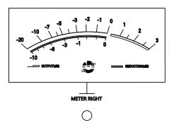
The meters provide information - optionally - on the magnitude of the signal level leaving the unit or the degree of interference from the compressor.
