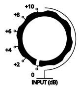
With the help of the input signal level controller, it is possible to increase the signal level entering the device if, for example, it does not reach the lowest interference threshold level, or if we want to achieve additional gain on the input for any reason. To adjust the input signal level, turn the control knob counterclockwise until the mark on the control knob points in the direction of the desired boost level.
