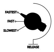
The RELEASE parameter determines how long it takes for the compressor to complete the intervention if the input signal level falls below the set intervention threshold level.
