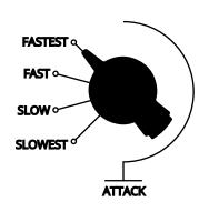
The sound we hear during compression is basically determined by the speed of the time constants, which in most cases will result from the nature of the program signal.
