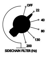
Depending on the program signal, it is often necessary for the dynamics controller not to react to deep frequency components. In such cases, it is advisable to filter out these low-frequency components from the auxiliary circuit signal controlling the compressor with a high-pass filter that does not allow a signal to the control circuit below a set cut-off frequency.
