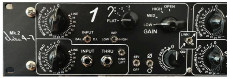
Intrument D.i. Input and Attenuator Pad.
