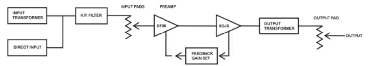
Tubes: EF86 input gain stage and 6DJ8 output driver.
