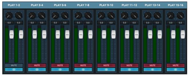
This pane is similar to the SD Play pane, but this is where streams from the computer are controlled. In many audio systems, the outputs you select in your audio software, are hardwired to go out specific outputs in the audio interface. That is not the case here. With Mesa, you have control over where these computer streams go, even if you want some playback material to go to multiple different outputs simultaneously.
