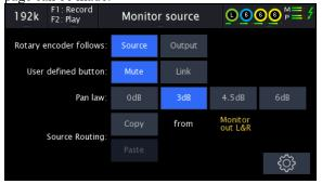
**Rotary encoder follows:** choose between Source or Output. Determines whether the rotary encoder controls the input source monitoring volume or the selected output volume from the Output Source page.
