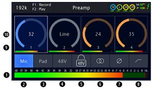
This page is where the four analog inputs can be controlled. You can select what type of input you wish to use, set input gain, link inputs, etc.
