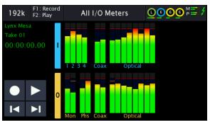
Mesa powers up to what is called the All I/O Meters page. This page is designed to reveal, at a glance, where there is signal present for the Mesa's inputs and outputs. The top row of meters represents inputs, and the bottom row outputs. In the default state, only the physicals ins and outs are represented here. The user can choose to have this page also reveal signals to and from the computer. This option is detailed in Section 3.2.5.
