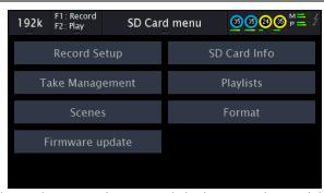
There are a few things going on here. The Mesa microSD card slot has several potential functions: Recording multichannel audio, saving and recalling user configuration "scenes", and performing firmware updates. All of these abilities are configured on this page.
