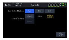
**User defined button:** allow selection of the controls to appear under the faders on the Outputs page. Mute is the default, Dim and Link are options
