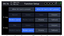
**Function Setup:** where the user can determine what the two Function buttons do when pressed. The user can choose what these operations will be with an SD card is present, or when an SD card is NOT present.
