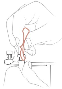
2. Remove the bottom suspension on the same side. Start at the larger mount point and slip the suspension pad over the rod and larger top mount point. Remove completely via the two outer, smaller mount points.
