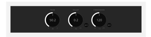
**Trim** - The first control is Trim, which raises or lowers the level of this speaker by up to 12dB, in increments of 0.1dB. Click and drag this control to either add or remove Trim from this speaker. Alternatively, double-click on the control to input a numeric value manually.
