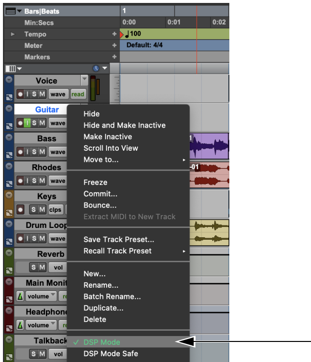
Right-click a track name to enable DSP Mode in the Edit window
