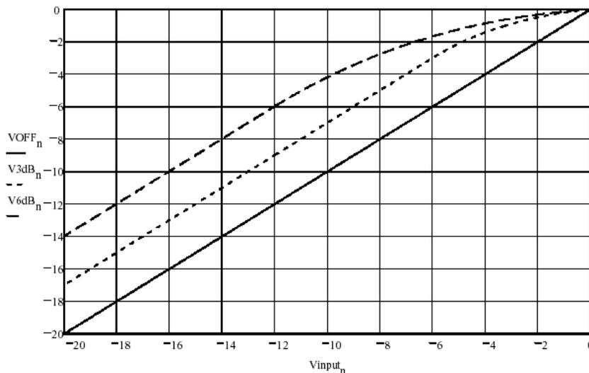
The algorithm for soft saturation is fundamentally different from classical audio compression. A compression algorithm provides time varying gain as a function of signal power. The gain variations are slowed down (attack and decay envelopes) to minimize distortions (a sudden step in signal gain generates a time decaying distortion).
